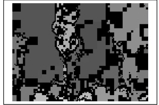
Fig. 2. The single depth intra mode areas of reconstructed depth map in gray color and other depth intra modes shown in black color on Figure 1.
