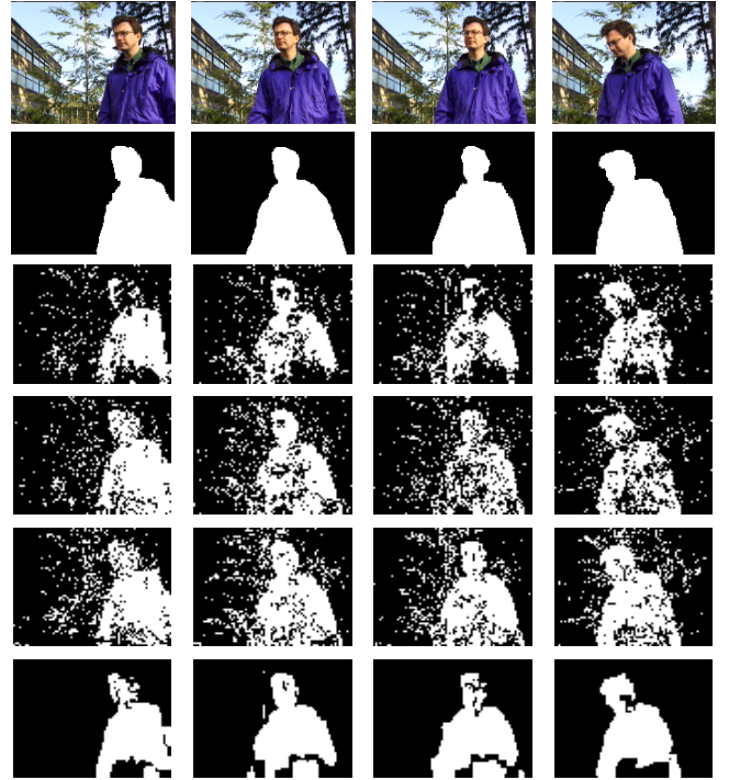
Fig. 2. Comparison results on the wavingtrees sequence. The top row is the original frames named as 245 th , 247 th , 251 th , and 254 th frames. The second row is corresponding ground truth frames. The third, fourth, and fifth rows are results obtained by the GMM, KDE, and Sparse methods respectively. The last row is the results obtained by the proposed method.
