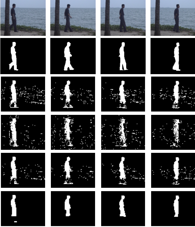
Fig. 3. Comparison results on the ripplingwater sequence. The top row is the original frames named as 1498 th , 1505 th , 1515 th , and 1526 th frames. The second row is corresponding ground truth frames. The third, fourth, and fifth rows are results obtained by the GMM, KDE, and Sparse methods respectively. The last row is the results obtained by the proposed method.
