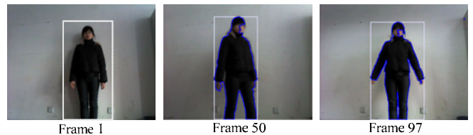
Figure 9. Object rough location and exact contour tracking in weak illumination scene for Zhang_2 video sequence.
