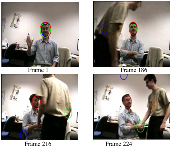
Figure 7. Anvar1GlobalNormal video sequence: Blue ellipse is the object tracking result from CPF; Green ellipse is the tracking result from CAMSGPF; And Red ellipse is the tracking result of our proposed.
