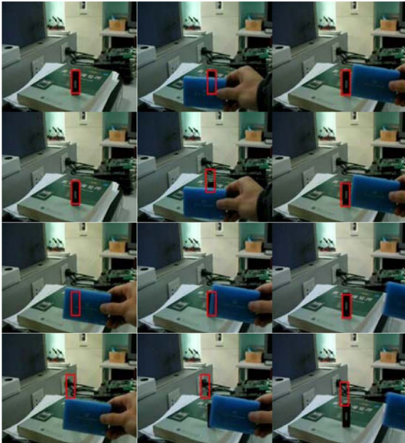
Figure 4. Occlusion adaptation of U-disk tracking results from OAPF (odd row) and CAMSGPF (even row). (frame 1, 106, 205, 216, 241, 248)
