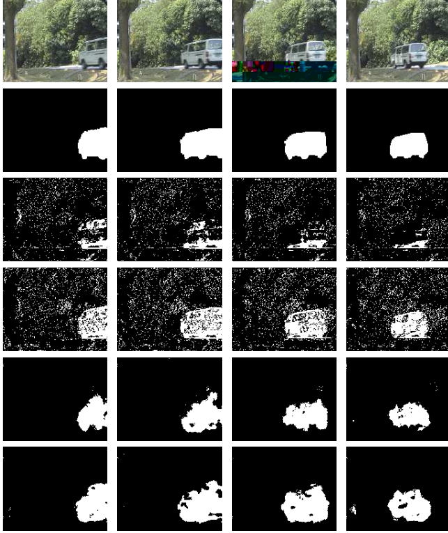
Fig. 5. Comparison results on campus sequence. The top row is the original frames named as 1202 th , 1204 th , 1206 th and 1208 th frames. The second row is corresponding ground truth frames. The third, fourth and fifth rows are the results obtained by GMM, KDE and LBP methods respectively. The last row is the results obtained by proposed method.
