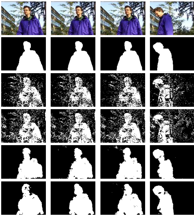
Fig. 3. Comparison results on waving trees. The top row shows the original 247 th , 249 th , 252 th and 256 th frames. The second shows are corresponding ground truth frames. The third, fourth and fifth rows are the results obtained by GMM, KDE and LBP respectively. The last row shows the results obtained by our approach. Note: Morphological operating are not used in the results.
