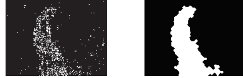
Fig. 1. Results before and after blob aggregation
