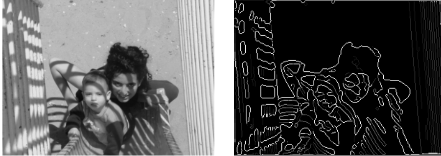
Fig. 1. Edges with different significance (global structures with long life-time in scale space are shown in high intensity and vice versa)
