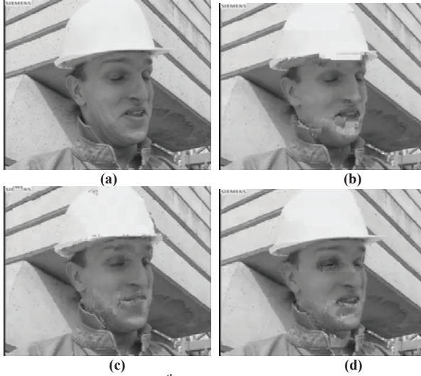
Fig. 4 The recovered 75 th frame of foreman with PLR = 20%, (a) no error frame (36.26dB) (b) no FMO mode (24.92dB), (c) chess pattern FMO (29.82dB), (d) proposed method (30.12dB).
