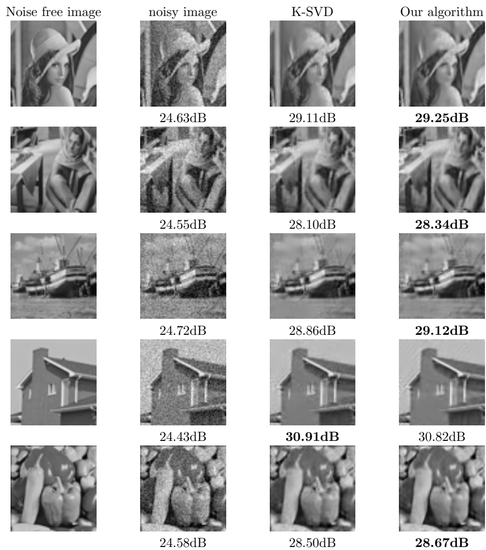
Figure 3. Original image, noisy image, denoised image of K-SVD and our proposed algorithm( \sigma = 15 ).
