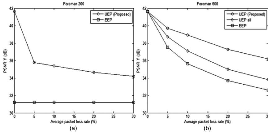
Fig. 2 PSNR comparison of the UEP scheme against EEP scheme for MGS enhancement NAL units.
