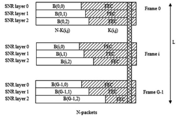
Fig. 1 UEP scheme for MGS enhancement NAL units in a GOP.
